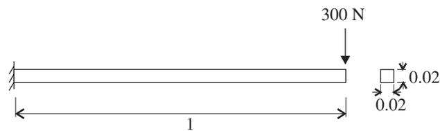
All lengths in meters. Step load applied at time 0.0.
