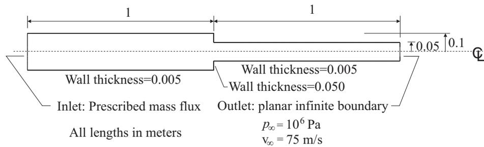
The fluid material properties are  $\rho = 1000 \text{ kg/m}^3$ ,  $\kappa = 2.1 \times 10^9 \text{ Pa}$ , and the solid material properties are  $E = 2.07 \times 10^{11} \text{ Pa}$ ,  $\nu = 0.3$ ,  $\rho = 7800 \text{ kg/m}^3$ .
