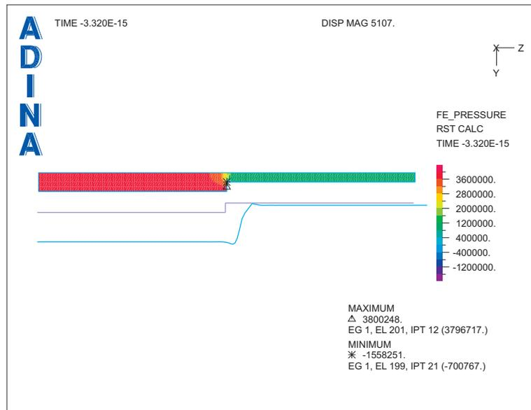
The pressure is higher at the inlet because the velocity is lower. In fact, the inlet and outlet pressures and velocities satisfy the Bernoulli equation  $\left(\frac{p}{\rho} + \frac{v^2}{2}\right)_{inlet} = \left(\frac{p}{\rho} + \frac{v^2}{2}\right)_{outlet}$ .
