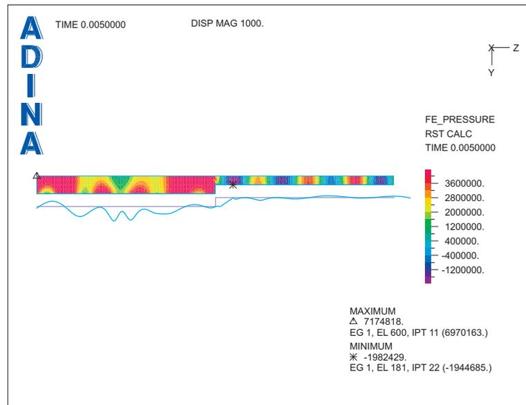
To animate the solution, choose Display→Movie Shoot→Load Step, set the Start Time to 0.0 and click OK. Pressure waves move from the inlet to the outlet. Eventually a standing wave pattern forms in the wide area of the pipe, because of reflections off of the constriction. However the waves always travel towards the outlet in the narrow area of the pipe, because of
