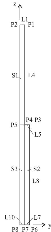
The model is defined in the y-z plane because the 2D potential-based elements and the axisymmetric shell elements must be defined in the y-z plane.
