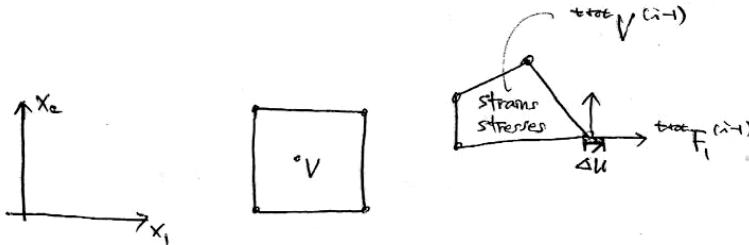
$${}^{t+\Delta t}K_{11}^{(i-1)} = \frac{\Delta \left({}^{t+\Delta t}F_1^{(i-1)}\right)}{\Delta u} \quad (18.22)$$
