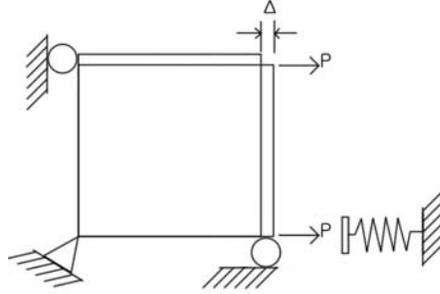
These are difficult to solve. The boundary conditions change when  $P$  is large to make the element take contact with the spring. The cases II to V may contain nonlinearities (a system could have combinations). Dynamic analysis can also be included in the system analysis.
